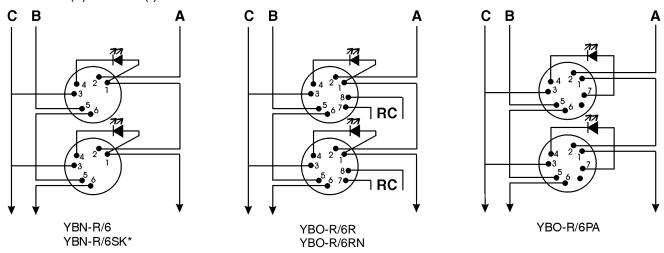
RC Relay Contacts - a flying lead on either terminal 7 or 8 selects either N/C or N/O (supplied as N/C)
